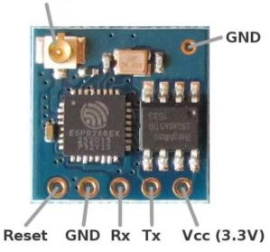
The 5pin version of the ESP8266 ESP-05 Serial WIFI Module has the following connections on the 5pin header:
