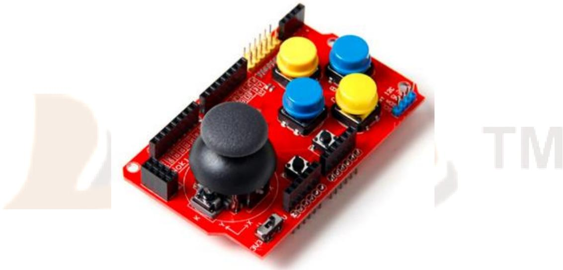
This JoyStick Shield Module Robotics Control is an Uno compatible shield that allows you to turn an Arduino Uno or compatible into a game console or robotic controller. 3.3V to 5V Gamepad Joystick Shield Module Game Rocker Button Controller Expansion Board For Arduino Simulated Keyboard Mouse Module.
