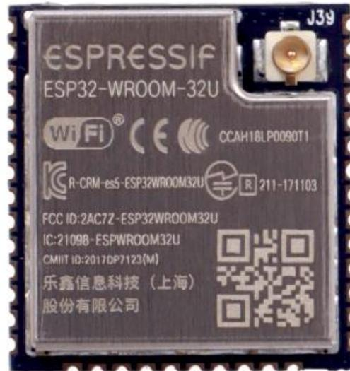
ESP32-WROOM-32U is powerful, generic Wi-Fi+BT+BLE MCU modules that target a wide variety of applications, ranging from low-power sensor networks to the most demanding tasks, such as voice encoding, music streaming and MP3 decoding.
