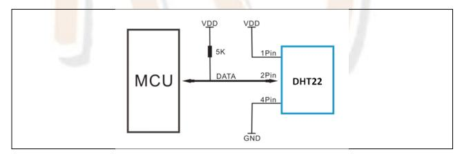
• As you can see the data pin is connected to an I/O pin of the MCU and a 5K pull up resistor is used. This data pin outputs the value of both temperature and humidity as serial data.
