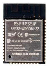
This is ESP WROOM 32 MCU Module. ESP WROOM 32 is a powerful, generic WiFi-BT-BLE MCU module that targets a wide variety of applications, ranging from low-power sensor networks to the most demanding tasks, such as voice encoding, music streaming, and MP3 decoding.
