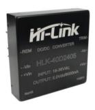
The output power of 40w DC to DC module power supply is 40w. 2:1 wide voltage input range, efficiency upto 91%, 1500Vdc isolation voltage, allowable operating temperature -40°C to +85°C, with output over voltage, over current, short circuit protection functions, bare metal meets CISPR32/EN55032 CLASS A, widely used in medical, industrial control, electrical power, instrumentation, communication, railway and other fields.
