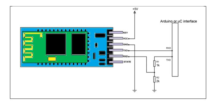
• Here the module is connected to +5V standard regulated power supply and UART interface is established as shown in figure. All you need to do is connect RXD of arduino
